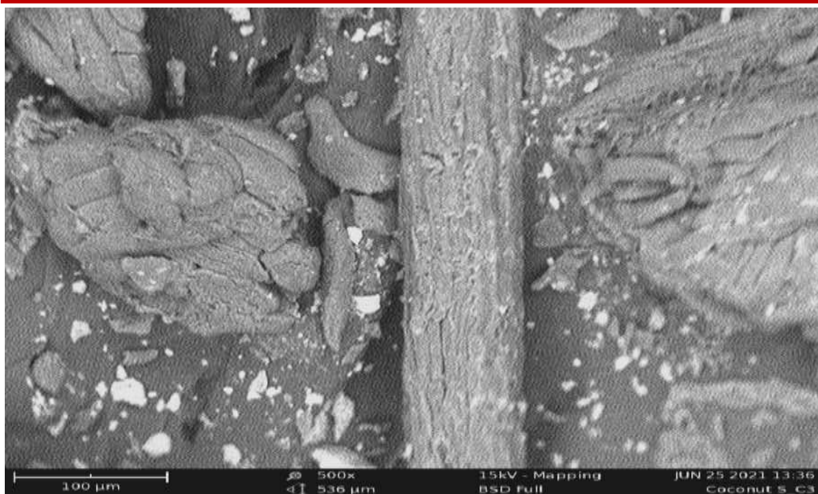
Figure 3.5: SEM image of coconut shell membrane (column 3) after filtration
